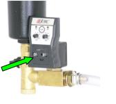
5. Place the connector gasket on the connector and plug the connector on to the timer as illustrated below and tighten the screw (max. 1Nm). Make sure both gaskets are secured properly to ensure IP65 rating.
